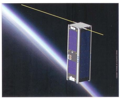
Besides being tested on the International Space Station, MSU's radiation-tolerant computer may eventually orbit the Earth as a stand-alone satellite.
