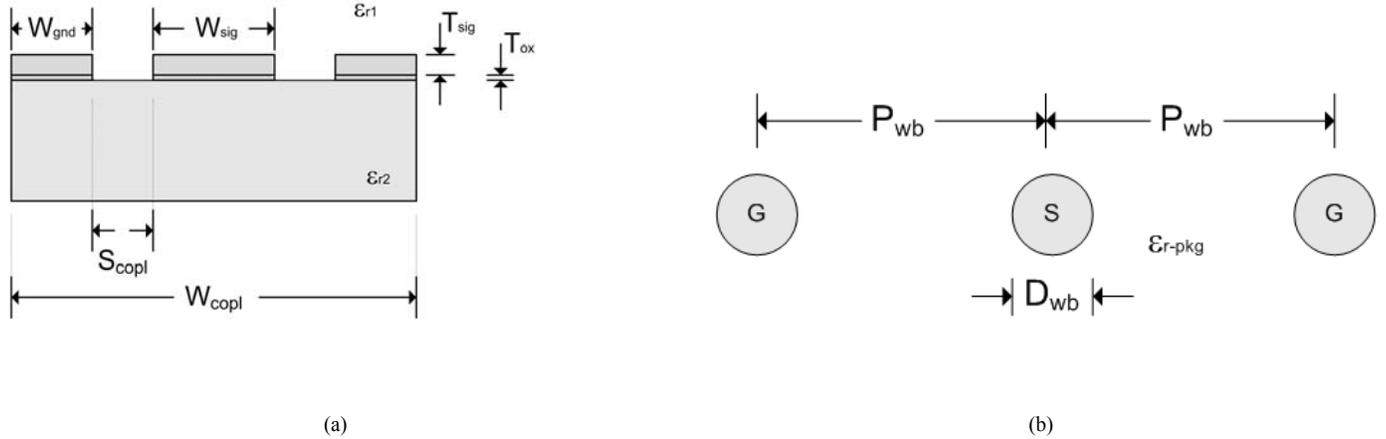
Fig. 2. Critical dimensions for the on-chip coplanar traces (a) and the off-chip coplanar wire bond (b) structures.
