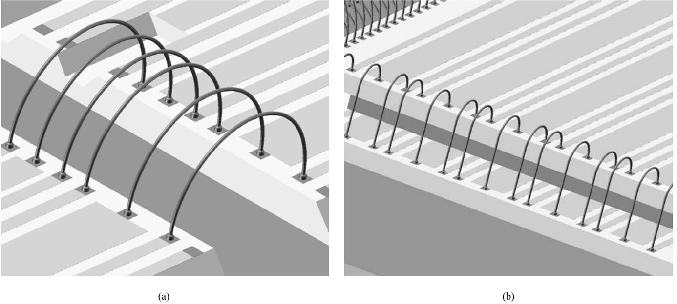
Fig. 1. 3-D Rendering of our interconnect approach used in an SiP application with adjacently-placed dies (a) and stacked-dies (b). Coplanar transmission lines on the two dies are connected using a G-S-G wire bond configuration.
