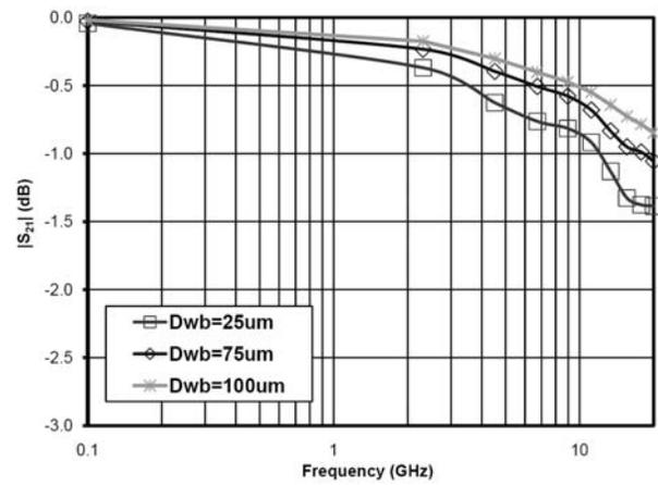
Fig 7.  $|S_{21}|$  response for the 75 $\Omega$  system with Gold wire bonds
