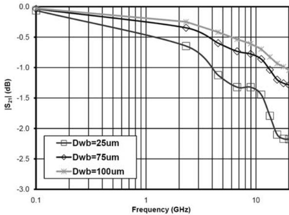
Fig 4.  $|S_{21}|$  response for the 50 $\Omega$  system with Aluminum wire bonds
