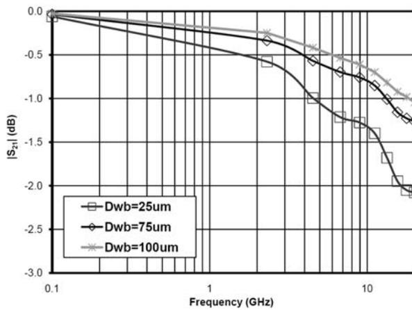
Fig 6.  $|S_{21}|$  response for the 50 $\Omega$  system with Gold wire bonds
