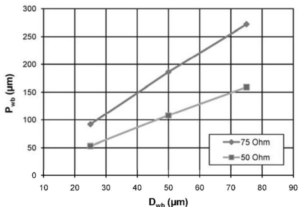
Fig. 3. Pitch vs. Diameter for the controlled impedance coplanar wire bond structure showing both a  $50\Omega$  and  $75\Omega$  system.
