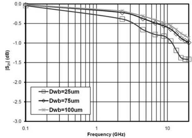
Fig 5.  $|S_{21}|$  response for the 75 $\Omega$  system with Aluminum wire bonds
