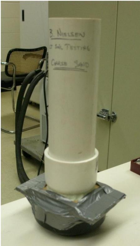
**Figure 6. 2" PVC pipe and platform.**
