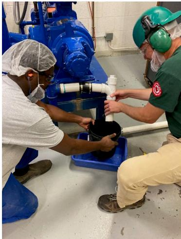
Figure 11: Filling bucket with discharge water in 10 seconds
