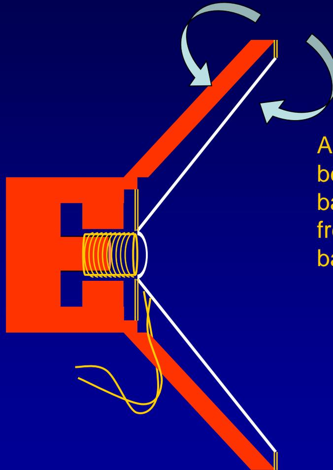
Air has time to “slosh” between front and back at low frequencies: poor bass response
