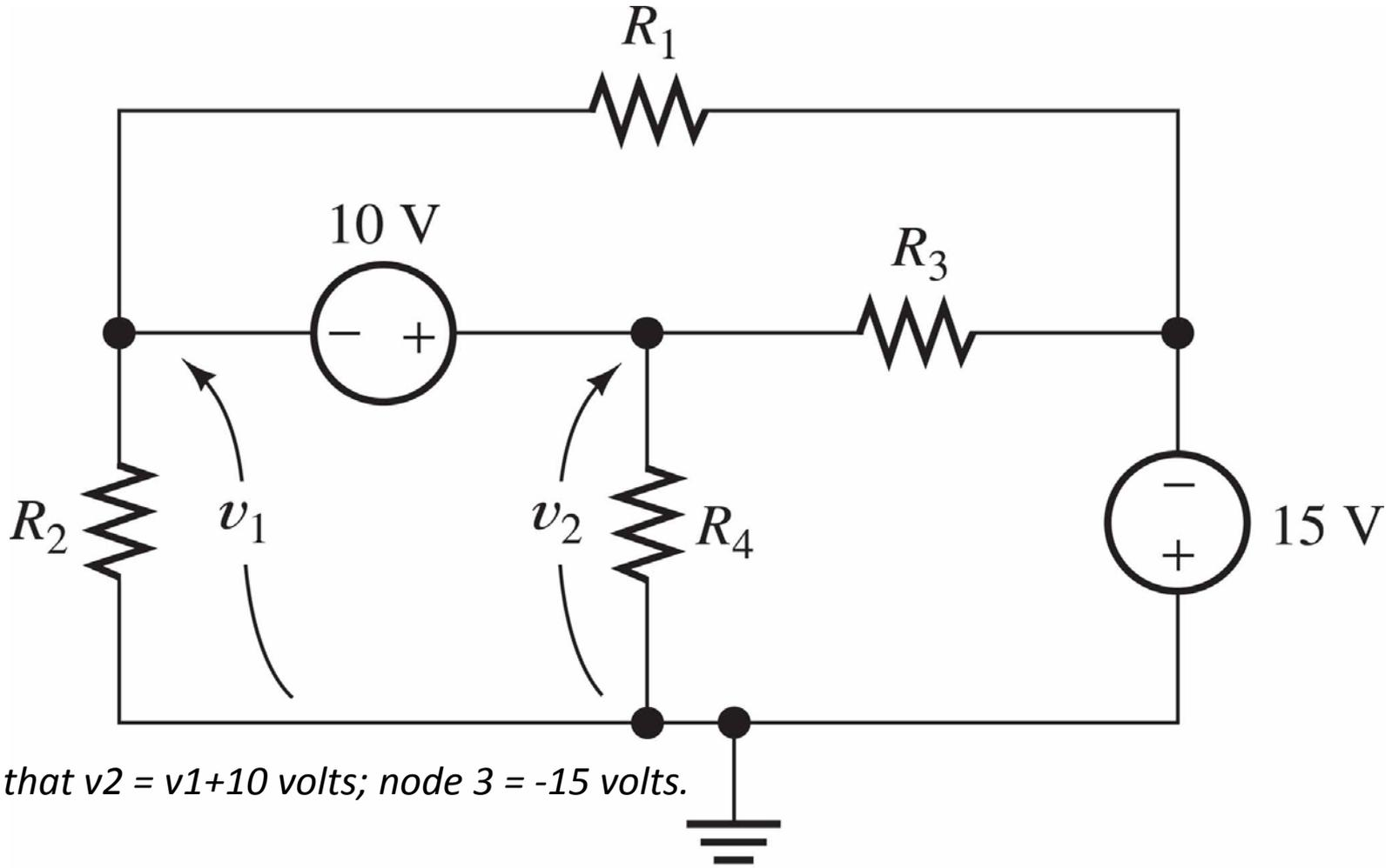
*Note that  $v_2 = v_1 + 10$  volts; node 3 = -15 volts.*
