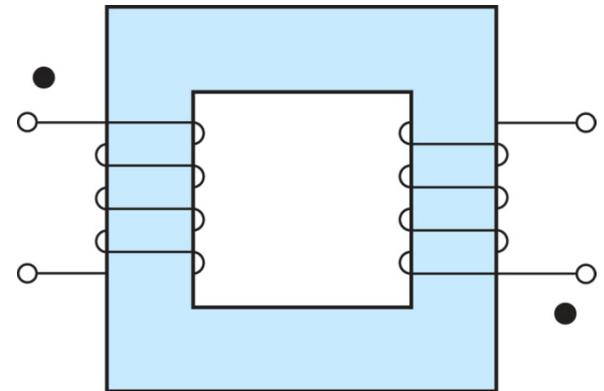
Dot labels: currents entering at the dots produce aiding fluxes
