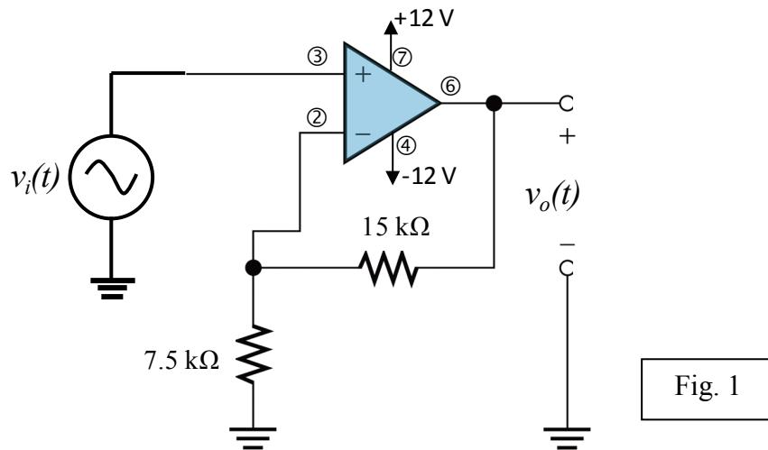
4. Using the oscilloscope to view  $v_i(t)$  on Ch 1 and  $v_o(t)$  on Ch 2, record the output voltage amplitude for each of the input sinusoid amplitudes in Table 1. Also calculate the voltage gain ( $|v_o|/|v_i|$ ) and list it in column 3 of the table.
