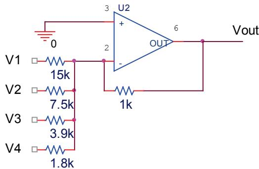
This circuit in Fig. 2 is a crude 4-bit “digital to analog converter,” meaning that if we treat V1 - V4 as binary digits (ones and zeros), the output voltage is proportional to the binary interpretation of those bits. Measure and record the output voltage for the following sequence of input voltage combinations shown in Table 2.
