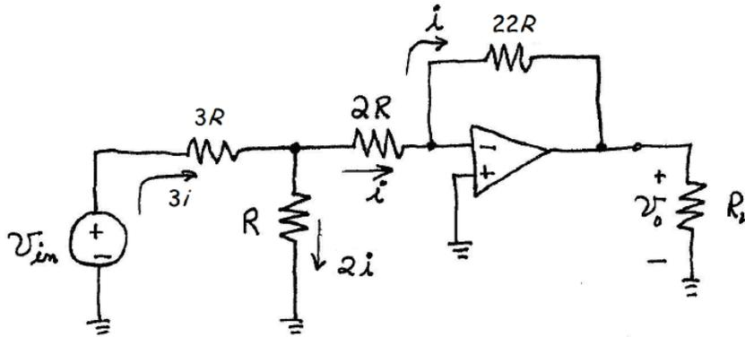
Applying KCL, we find the other currents as shown. Then, applying KVL, we have  $v_{in} = 3R(3i) + 2Ri$  and  $v_o = -22Ri$ . Solving, we find  $A_v = \frac{v_o}{v_{in}} = -2$ .
