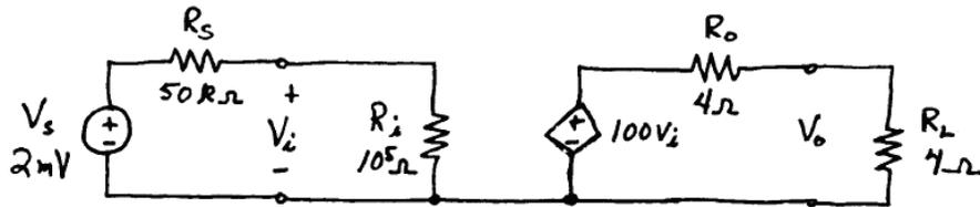
$$A_v = \frac{V_o}{V_i} = A_{oc} \frac{R_L}{R_o + R_L} = 100 \frac{4}{4 + 4} = 50$$
