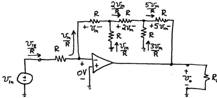
From these results we can use KVL to determine that  $v_o = -8v_{in}$  from which we have  $A_v = -8$ .
