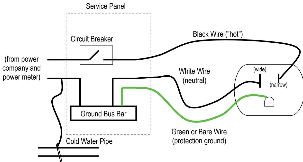
The “ground” connection from the incoming power line is connected to a buried ground rod or tied to a metal water pipe as close to the entry point as possible. The only purpose for this literal ground attachment is lightning protection. When lightning hits the power pole, the lowest impedance return to earth ground is through this connection--and not through the premises!
