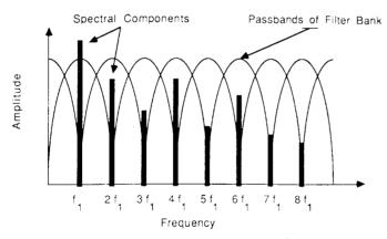
**Fig. 1.** A fixed-band harmonic analyzer employs a bank of bandpass filters centered at the harmonic frequencies. Vibrato causes the spectral components to shift back and forth in frequency, resulting in a misalignment ('cross-talk') between the analysis filters.
