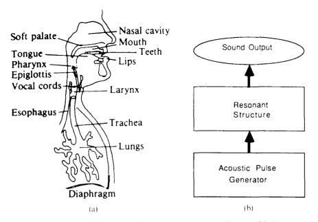
**Fig. 4.** A schematic model for the vocal apparatus. (a) Cutaway diagram of the human vocal system (after Rossing *et al.*<sup>9</sup>). (b) Simple block diagram consisting of an acoustic pulse generator (lungs and vocal cords) and a resonant structure (pharynx, oral cavity, etc.).
