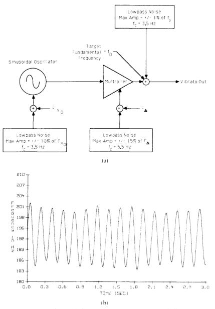
**Fig. 11.** Block diagram for vocal vibrato simulation. (a) The nominal vibrato rate  $f_{x_0}$  and depth  $f_{\Delta}$  vary in a quasi-random manner. A low-frequency drift of the target fundamental is also present. (b) Example of vibrato waveform generated by the process in (a).
