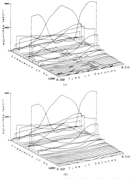
**Fig. 5.** Example of the conversion from a full MQ analysis to quasi-harmonic form. (a) A portion of the MQ analyzer output for a sung tenor tone. (b) The example of (a) following quasi-harmonic extraction based on fundamental frequency tracking.
